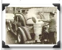
known as producer gas. The gas was then fed into the engine to generate power and propel the vehicle. This process, known as gasification,
